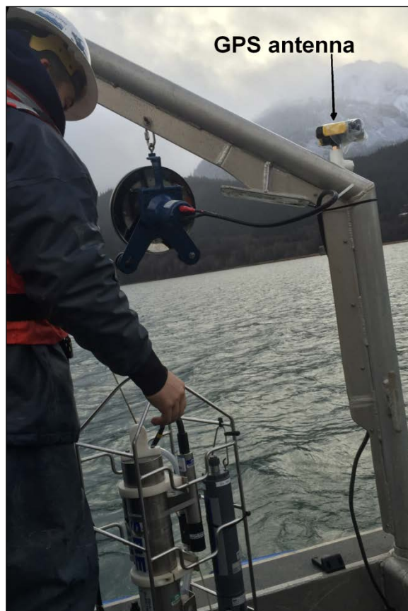
Figure 1. GPS Antenna Mounted with an Offset from the Winch Location
